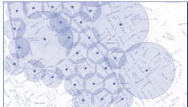
Fig. 8. Smaller cells accommodate more cell phones per unit area. Larger cells cover low traffic areas.
